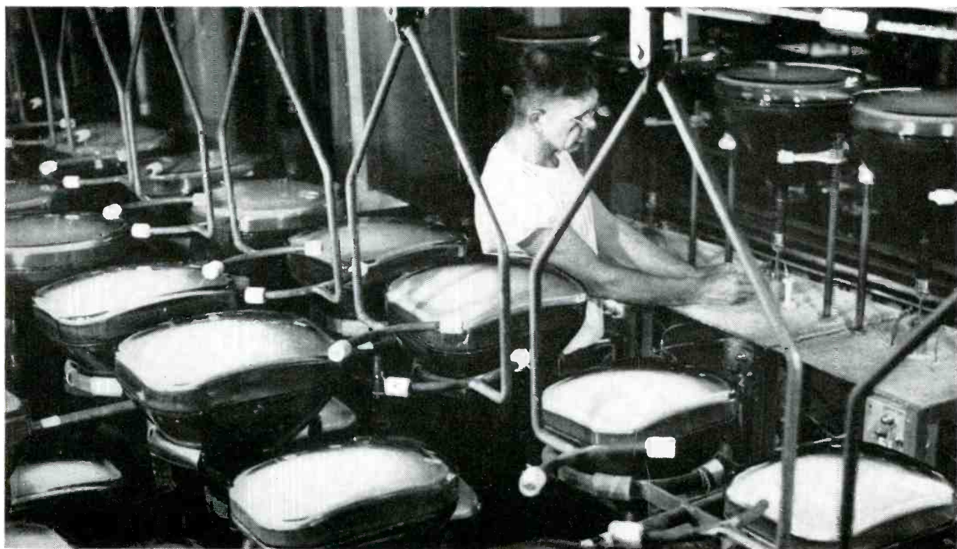
Loading dollies for the picture tube exhaust oven.
